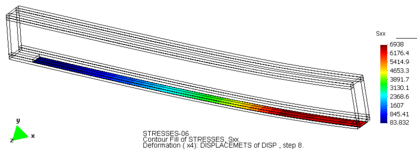
Figure 2.25: Stress state in CFRP reinforcement. Sp3D-R1 model
