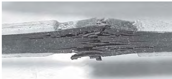
Figure 3.1: Delamination due to compression in a carbon/epoxy composite (Paiva et al., 2005)
