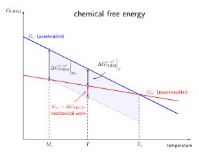
Fig. 5 Martensitic transformation. Energies involved.
