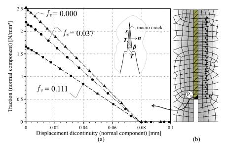
Fig. 12 Single-Edge Notched Beam Test with inner heterogeneous microstructure. Homogenized cohesive responses  $(T_n \text{ vs.} \beta_n)$  obtained using the Failure-Oriented Multi-Scale Formulation. Curves evaluated at point P<sub>II</sub> (see picture-(b)), for different void volume fractions.
