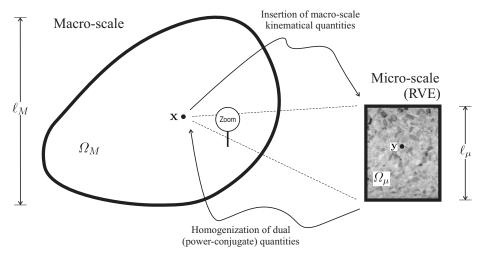
Fig. 2 RVE-based multiscale modeling. The RVE concept.
