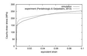
Fig. 8 Stress-strain response under monotonic shearing.
