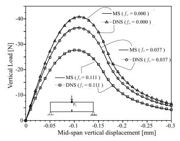
Fig. 11 Single-Edge Notched Beam Test with inner heterogeneous microstructure. Vertical load vs. vertical displacement curve for point  $P_I$ . Comparison between MS and DNS approaches for different void volume fractions.
