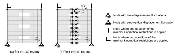
Fig. 10 Single-Edge Notched Beam Test with inner heterogeneous microstructure. RVE kinematical restrictions. (a) Standard Boundary Conditions for the stable macroscopic regime  $(t < t_N)$ . (b) Non-Standar Boundary Conditions for the unstable macroscopic regime  $(t > t_N)$ .
