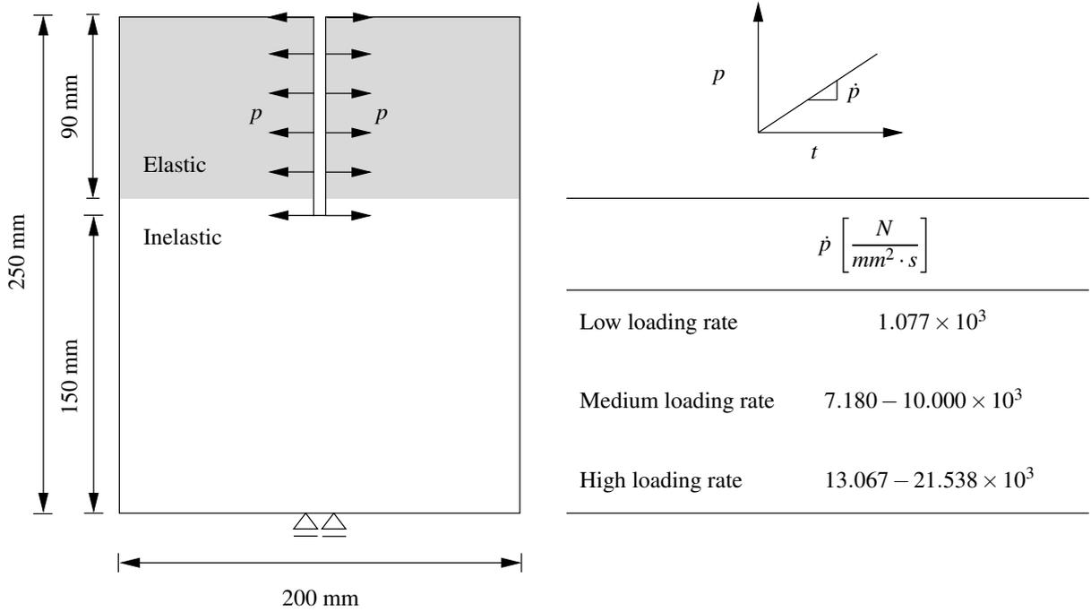
Figure 4: Geometry and boundary conditions for the dynamic CT test.
