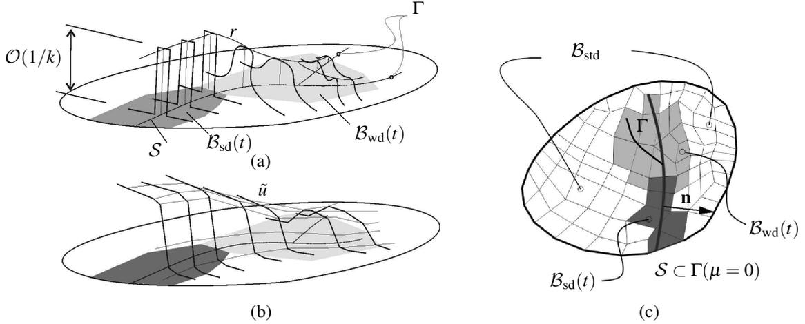
Figure 3: Crack Path Field (CPF) strategy for the crack tracking algorithm.  $\Gamma$  denotes the crack path set. (a) Localized field  $r$  around a strong discontinuity band. (b) Associated scalar displacement field  $\tilde{u}$ . (c)  $\Gamma$  (zero-level set of the crack path field function  $\tilde{\mu}$ ) and the trace of the strong discontinuity  $\mathcal{S}$ .
