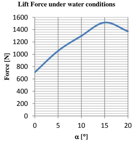
**Fig 12. Numerical lift force obtained under water conditions**
