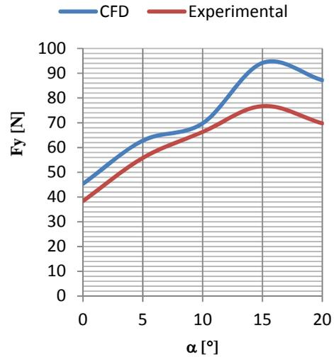
**Fig.7 Lift force generated by airfoil in air fluid conditions**
