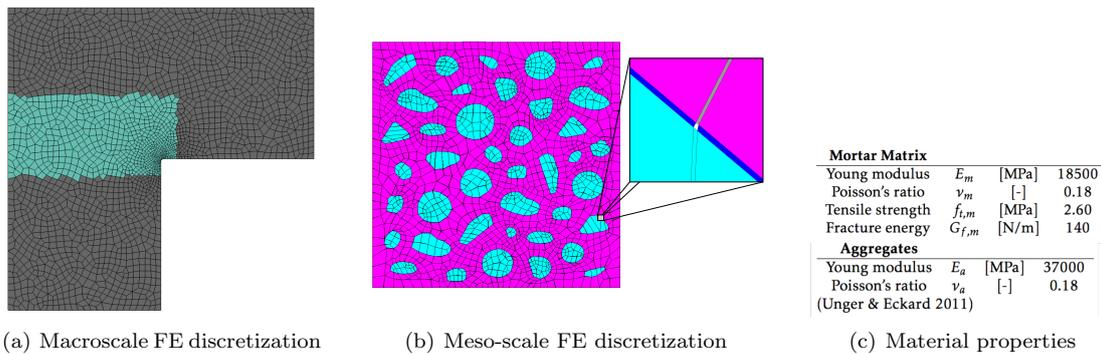
Figure 1: Finite element discretization and material properties
