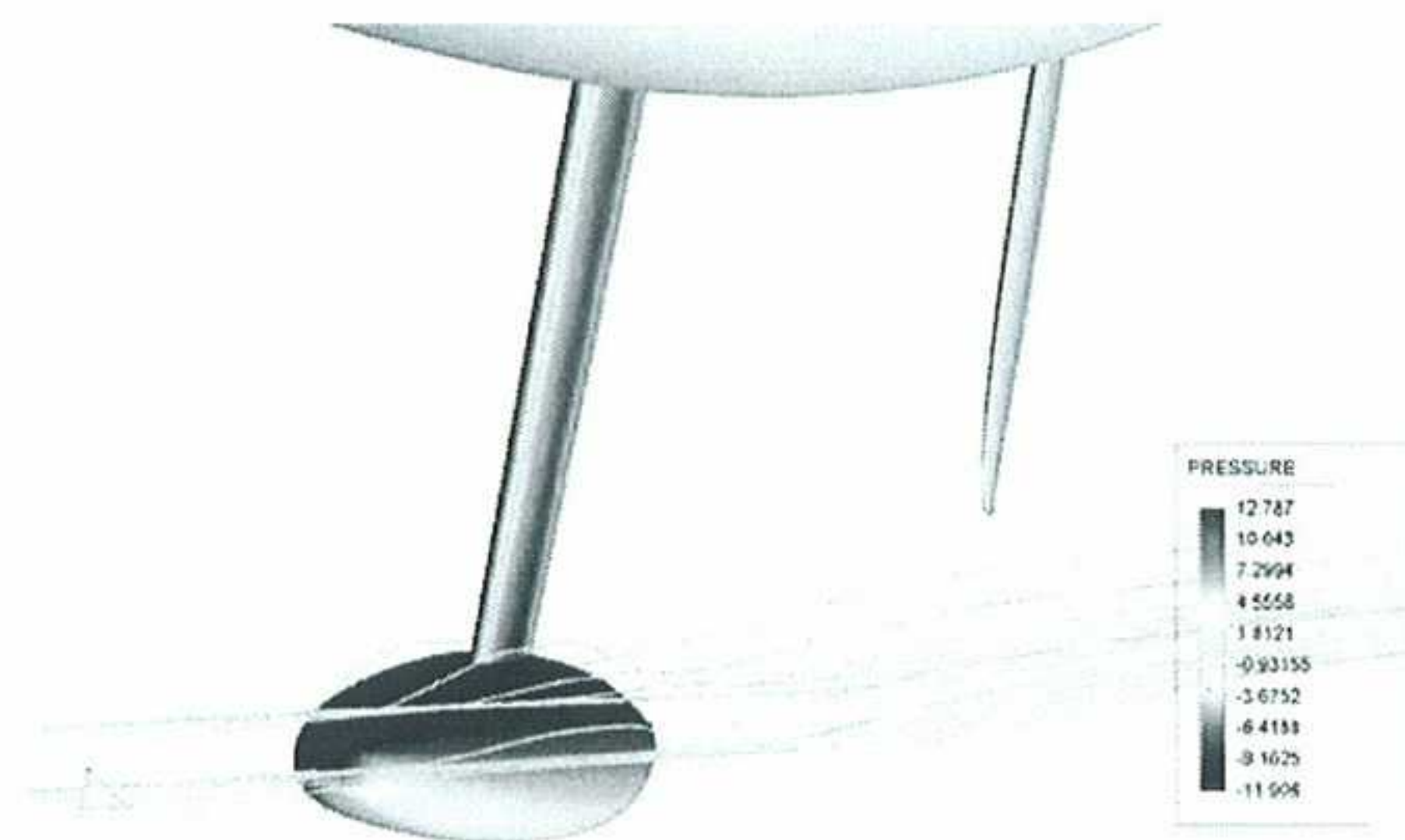
Figure 20. E15D2 7.5 kn. Pressure map on appendages and streamlines. Perspective view
